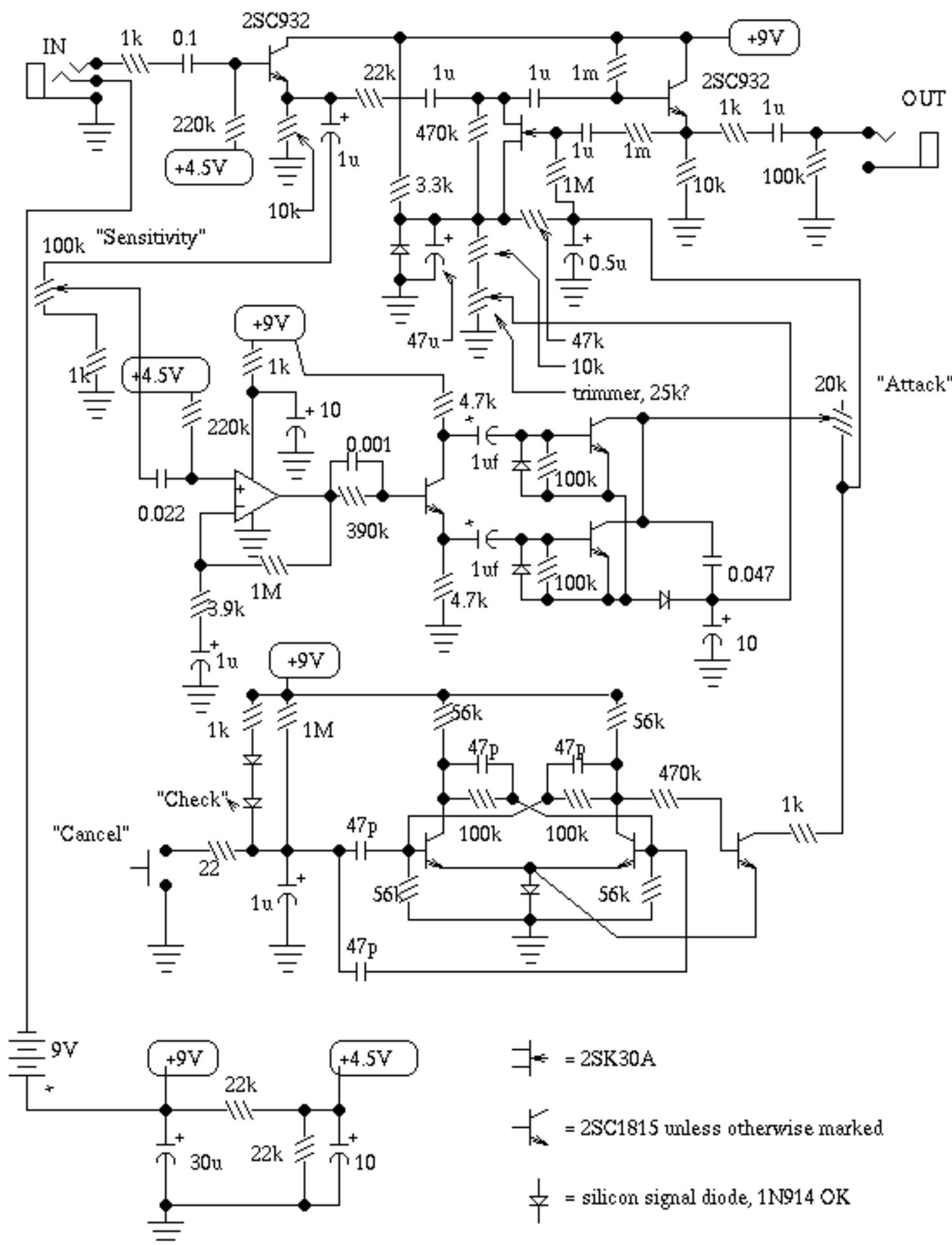
The SG-1 is an attack delay unit. A struck note is at first inaudible, then fades up, similar to a reversed tape recording.
