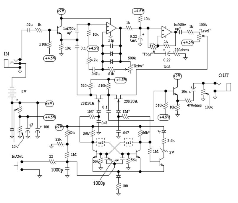
Opamps are in a dual 8 pin dip, 4558. All transistors 2SC1815. All diodes silicon signal diodes, 1n914 or similar. np\* = nonpolorized resistors denoted by \* marked as 1M on original might be 22k and those marked as 56K might be 10k. crf1 and cr2 are a special cap and resistor in parallel, the cap is 51p the resistor is 56k.
