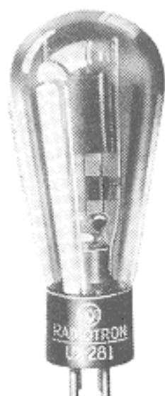
The '81 is a half-wave rectifier tube for use in d-c socket-power devices operating from the alternating current supply line. Full-wave rectification may be accomplished by two '81's.
