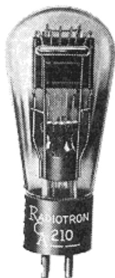
The type '10 is a three-electrode high-vacuum tube suitable for power amplifier use. As an audio-frequency amplifier, it is capable of delivering large undistorted output to the loudspeaker.
