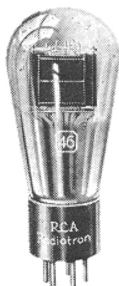
The '46 is a double-grid power amplifier tube recommended especially for service in Class B amplifier circuits of suitable design. In such circuits an output stage is preceded by a power amplifier stage designated as the "driver." A pair of '46's in a Class B output stage is capable of supplying an exceptionally large amount of virtually undistorted power; while a single '46, operated in the
